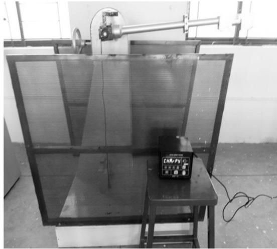
**Fig.3.**Experimental setup of the impact test.
