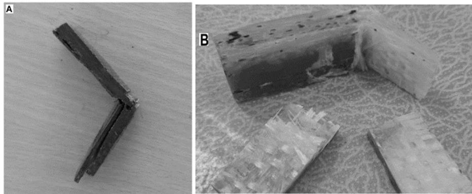
**Fig.5.**(A) Carefully constructed top view of the final CFRP test specimen. (B) The obtained GFRP test specimen seen from an isometric viewpoint.
