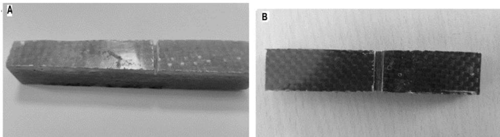
**Fig. 4.**(A) A representative top view of the test specimen made of GFRP. (B) An exemplary top view of the test specimen based on CFRP.
