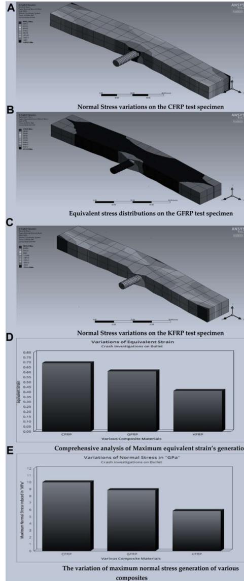
A thorough examination of the creation of the greatest equivalent strain. (E) Variation in different composites' maximum normal stress generation.
